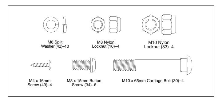
While another person lifts the front of the Frame (1) slightly, attach a Stabilizer (2) with two M10 x 65mm Carriage Bolts (30) and two M10 Nylon Locknuts (33).
